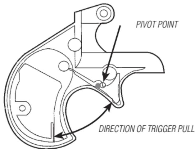
*The drawing above indicates the direction that the trigger should be pulled to allow the trigger to move in it's designed path (the path of lowest resistance). Pull in a downward motion toward the bottom of the gun. DO NOT pull straight back.*
